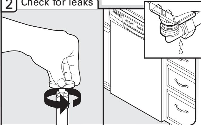
Place paper towel under 90° elbow fitting. Turn on water supply and check for leaks. If leak occurs, repeat previous step.
